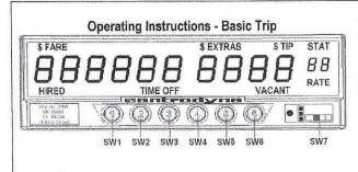
VACANT: The taximeter is normally in the Vacant state. If required, press switch 6 to select rate. Press switch 1 (SW1) to Hire taximeter.
