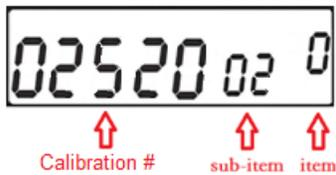
and KEY2 will no longer function. This is auto-calibration mode. Move the vehicle to the start point of a measured mile or km and stop, select the programming item to Calibration number, the previous stored Calibration number will show on the screen, move the vehicle and stop when a measured mile or km is reached, press KEY3 to save the new number into taximeter.
